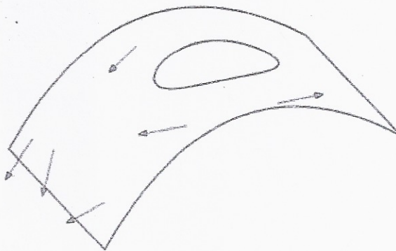
Fig. 3 Optimum gauge locations and orientations
