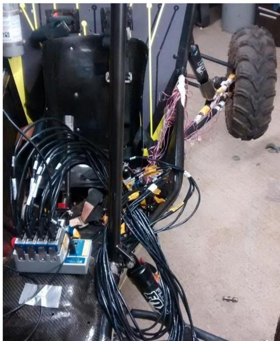
Figure 9. Instrumented vehicle with Data Acquisition System
