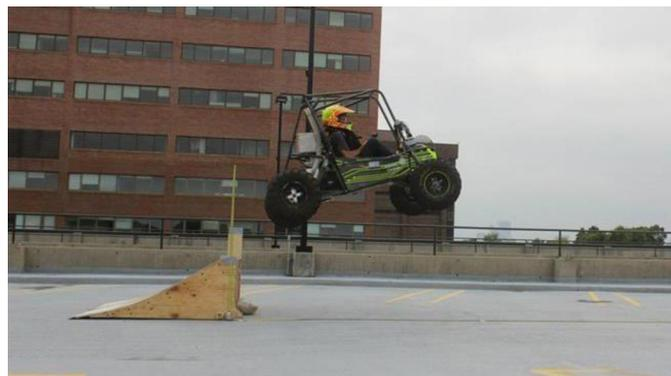
Figure 10. Instrumented vehicle under high jump testing, 10 mph
