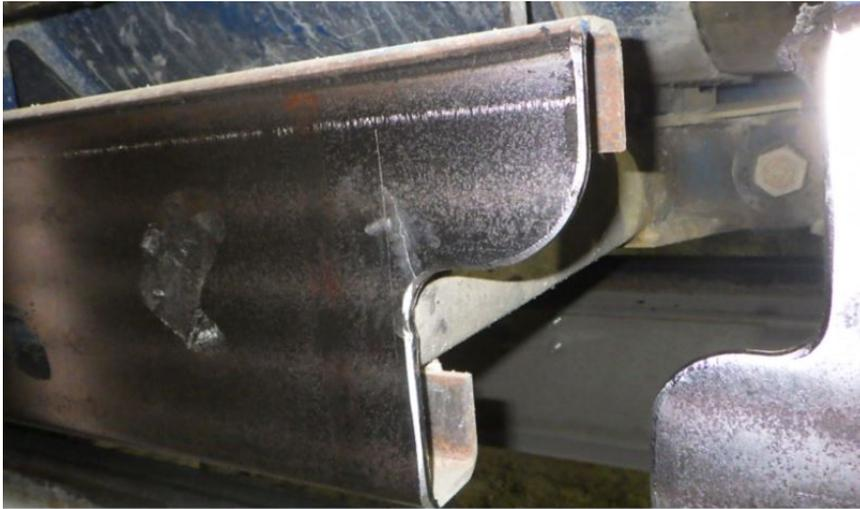
*Figure 3: Vertical Crack at front end of the side panel*
