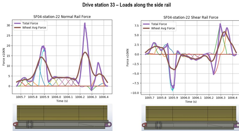
Figure 16: Normal and shear forces from the tire vs Time at drive station 33 - Train going down
