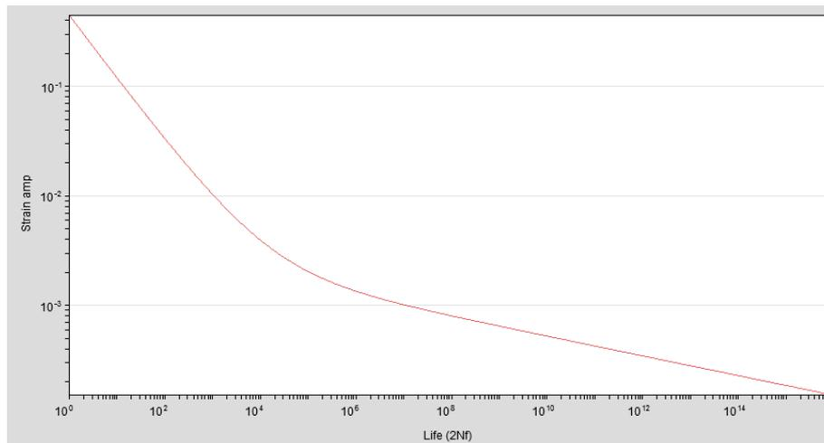
Figure 8: A572 Gr 50 strain life curve
