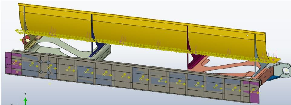
Figure 10: Unit loads definition for True-Load showing 14 concentrated force on the side rail
