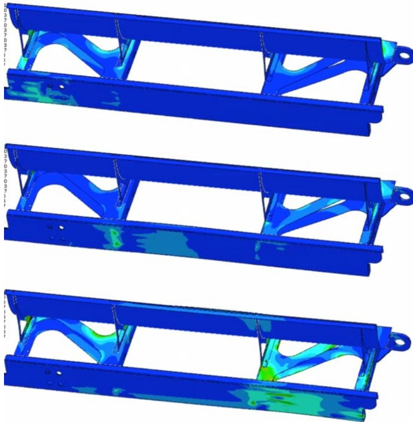
Figure 18: Snap shot of the sequence of stress results while the car goes through the drive station - using True-Load loading
