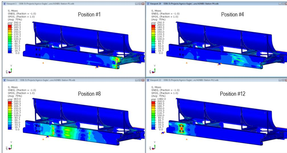
Figure 6: Von Mises stress (MPa) for tire loading at four (4) different positions along the car length
