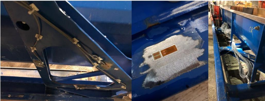
Figure 12: Strain gauges installation
