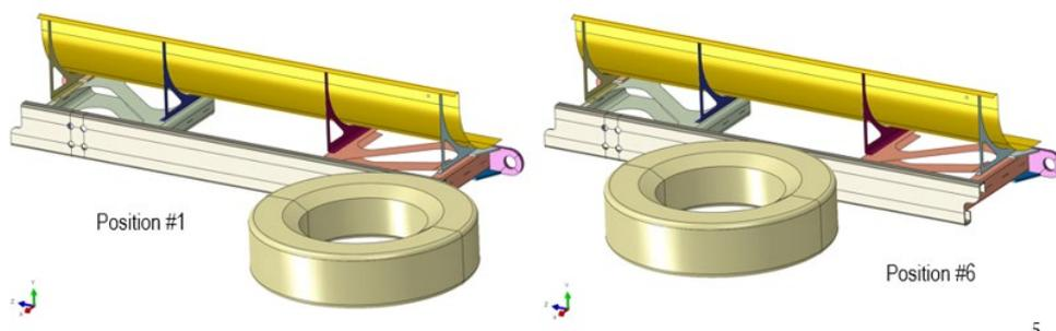
Figure 5: Static FE Model with two (2) different tire positions
