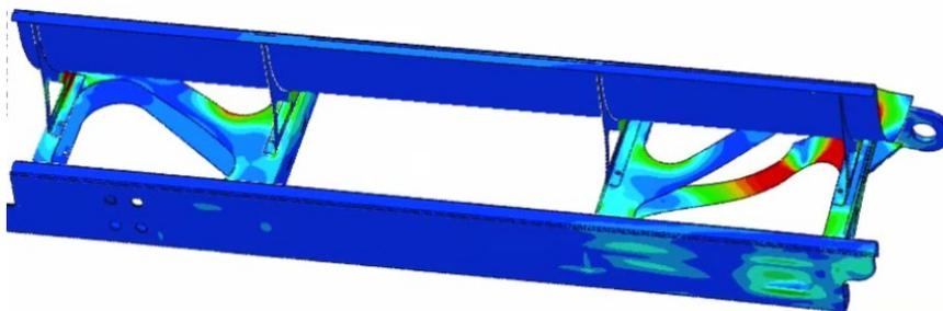
Figure 19: Stress results when tire is at the front of the car showing the front cross members buckling
