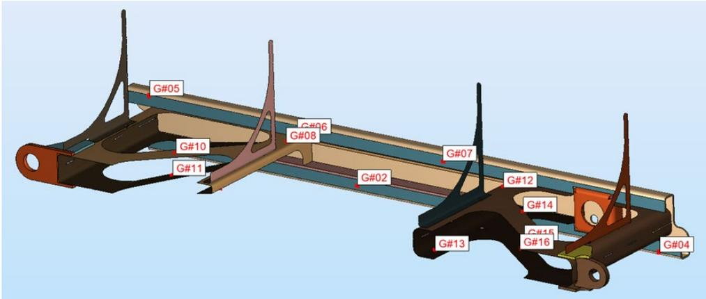
Figure 11: Strain gauges location as optimized by True-Load
