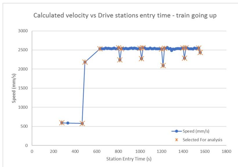
Figure 13: Average car velocity at each drive station (blue dot) while going up
