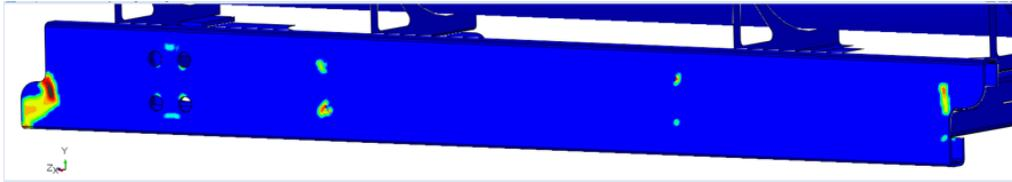
Figure 9: Log of Fatigue life for the 182 repeats of a drive station passage
