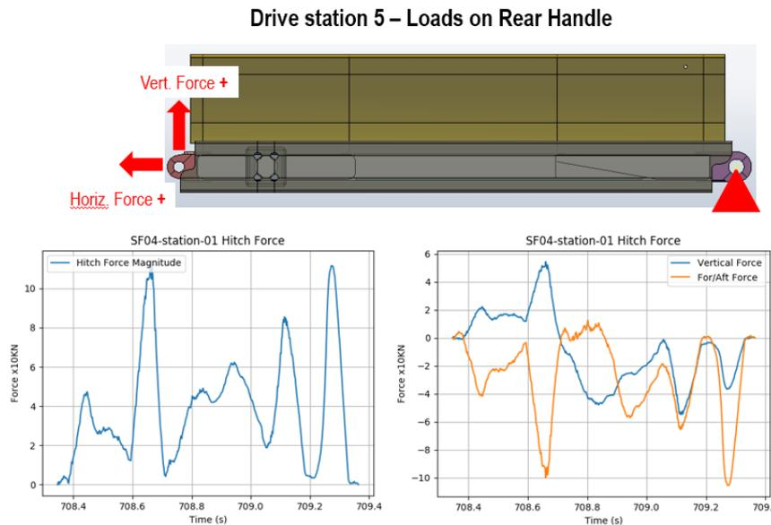
Figure 17: Horizontal and vertical forces on the rear handle at station 5 – Train going down
