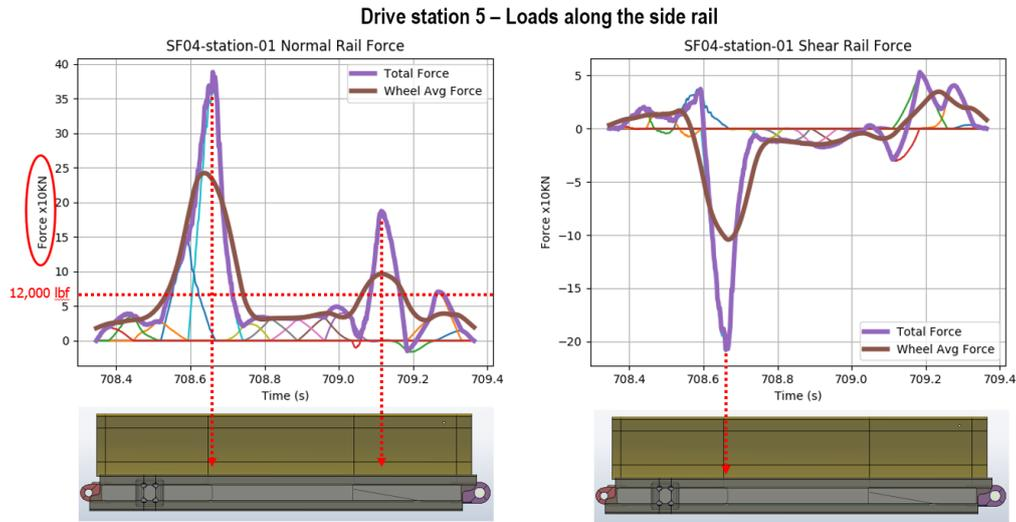
Figure 15: Normal and shear forces from the tire vs time at drive station 5 - Train going down
