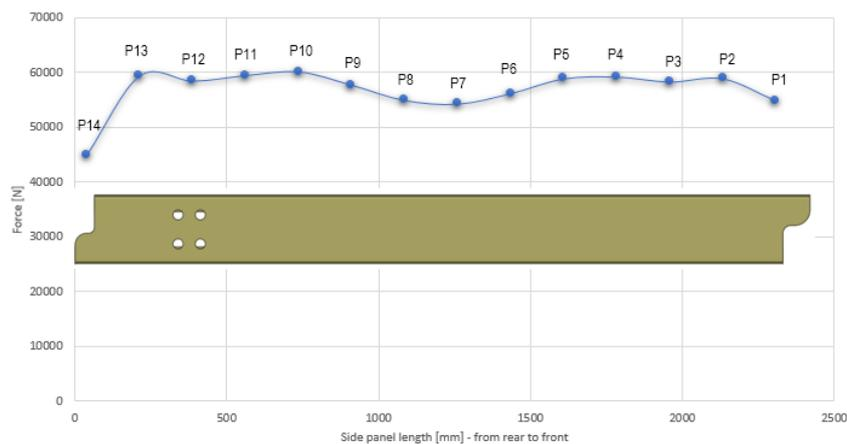
Figure 7: Tire reaction force for all fourteen (14) positions along the car length
