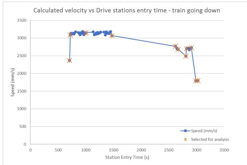
Figure 14: Average car velocity at each drive station (blue dot) while going down
