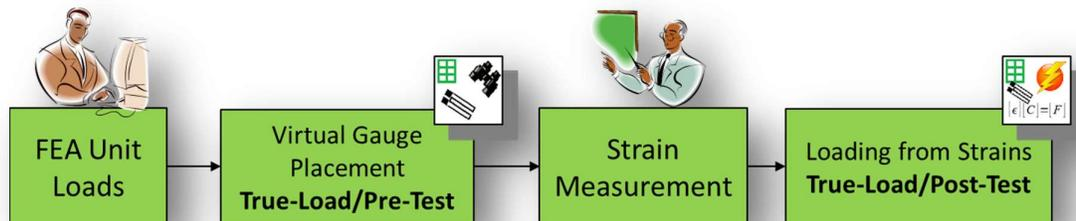
Figure 2: Load Reconstruction Process Schematic
