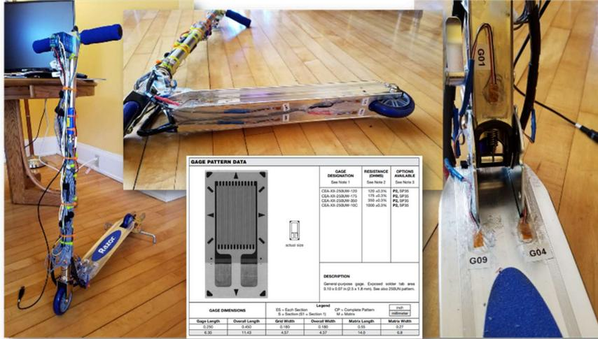
**Figure 5: Strain Gauge Placement**
