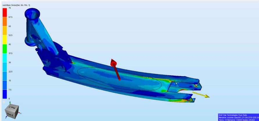
Figure 15: Typical Frame from a Reconstructed Operating Deflection Shape
