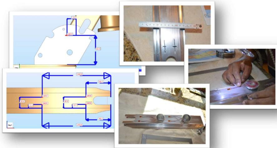
Figure 10: Strain Gauge Installation
