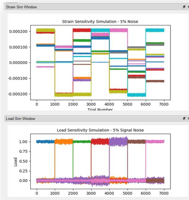
**Figure 9: Load Sensitivity to Strain Signal Noise**
