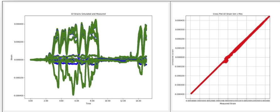
Figure 14: Overall Strain Correlation Plot
