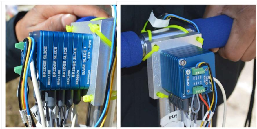
Figure 11: DAQ used for Strain Data Collection
