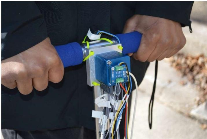
**Figure 4: DTS Slice Micro DAQ**
