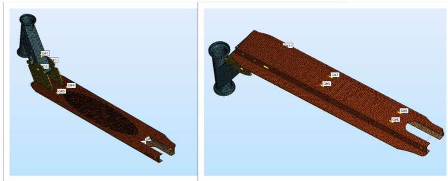
Figure 8: Virtual Strain Gauge Placement
