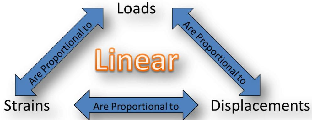
**Figure 1: Linear material behaviour schematic**
