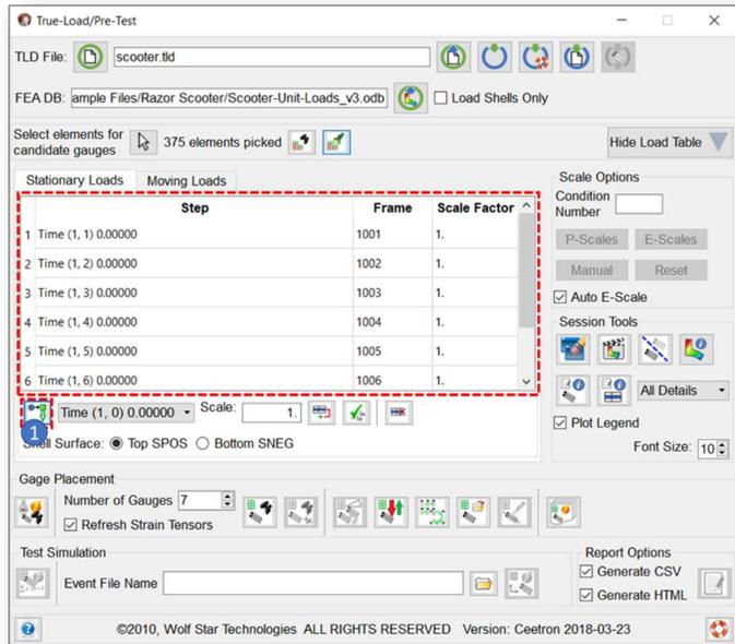
Figure 7: Pre-Test GUI with Load Table
