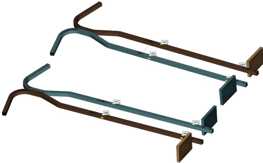
**Figure 4-8 Virtual Strain Gauge Placement**
