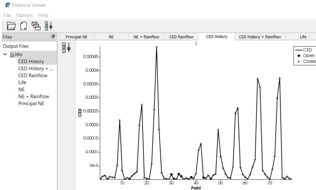
**Figure 6-7 Cracking energy density history on the critical plane in the most critical finite element. The crack open/close state is indicated by the symbols.**
