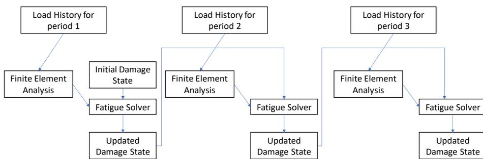
Figure 6-8 Incremental fatigue analysis workflow.
