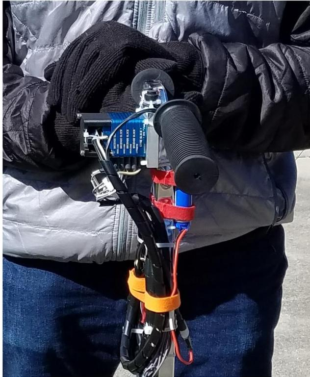
**Figure 4-4 DTS Slice Micro DAQ**
