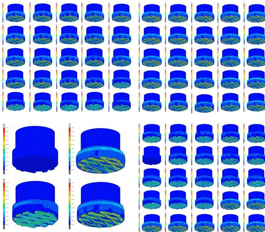
**Figure 6-2 Pogo stick rubber tip finite element model results for the 75 cases comprising the map. Each case represents a unique combination of vertical and side loads. Contours show maximum principal strain.**
