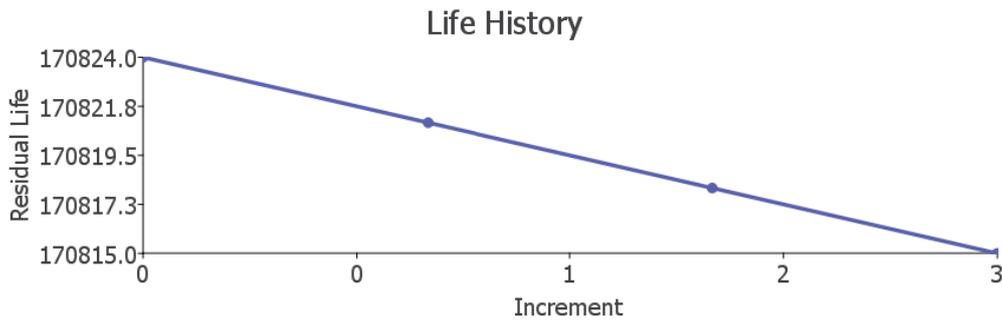
Figure 6-10 Development of residual life, measured in repeats of the standard load case, over 3 update periods.
