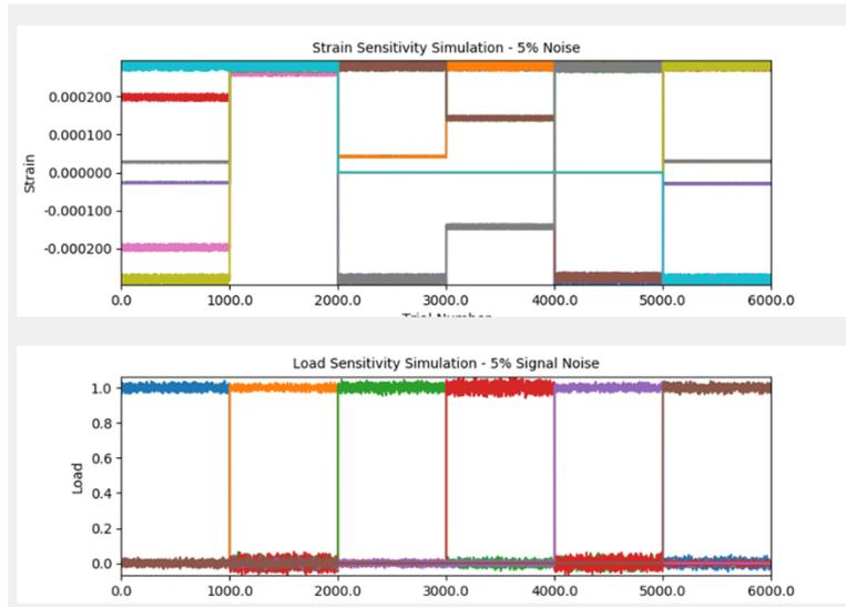
Figure 4-9 Load Sensitivity to Strain Signal Noise
