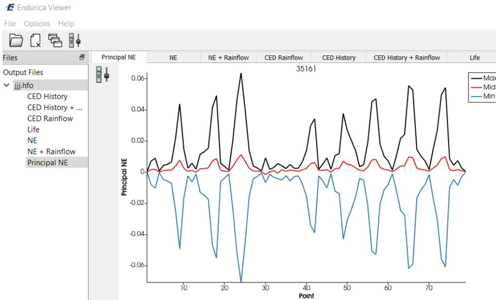
**Figure 6-6 Maximum principal engineering strain history in most critical finite element as solved via the interpolation process.**
