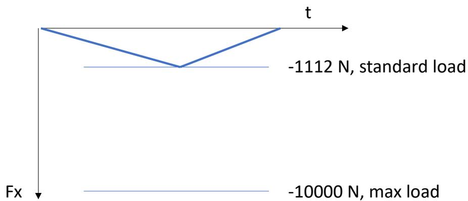
**Figure 6-3 Pogo stick standard load case. Residual life is reported as repeats of this load case.**
