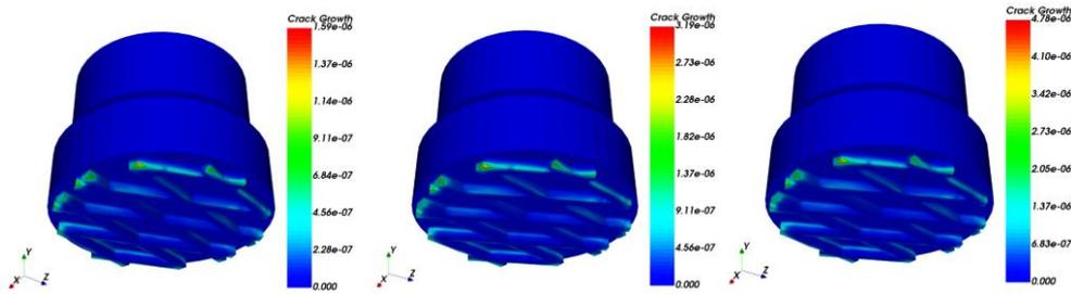
Figure 6-9 Crack precursor development over 3 update periods.
