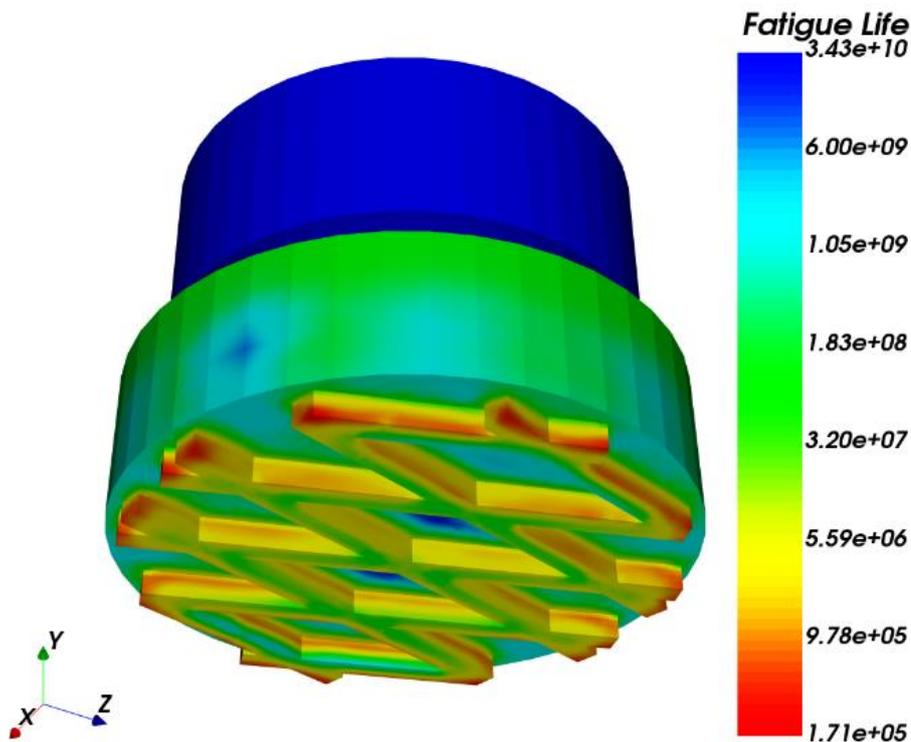
Figure 6-4 Initial distribution of residual fatigue life, given as repeats of the standard load case.
