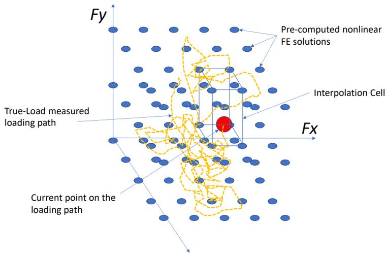
**Figure 6-1 Endurica EIE interpolation scheme. Nonlinear finite element solutions are pre-computed for each map point. The pre-computed solutions are used to interpolate the strain components at each element for the current point on the loading path, based on the solutions at the vertices of the interpolation cell.**
