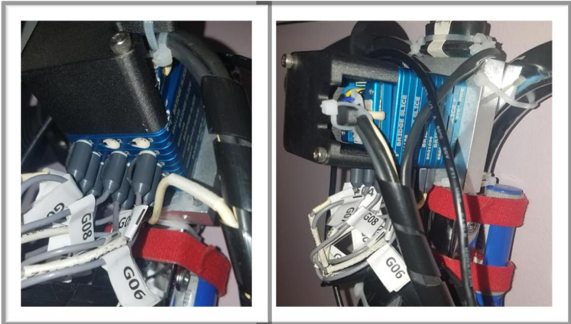
Figure 4-11 DAQ used for Strain Data Collection
