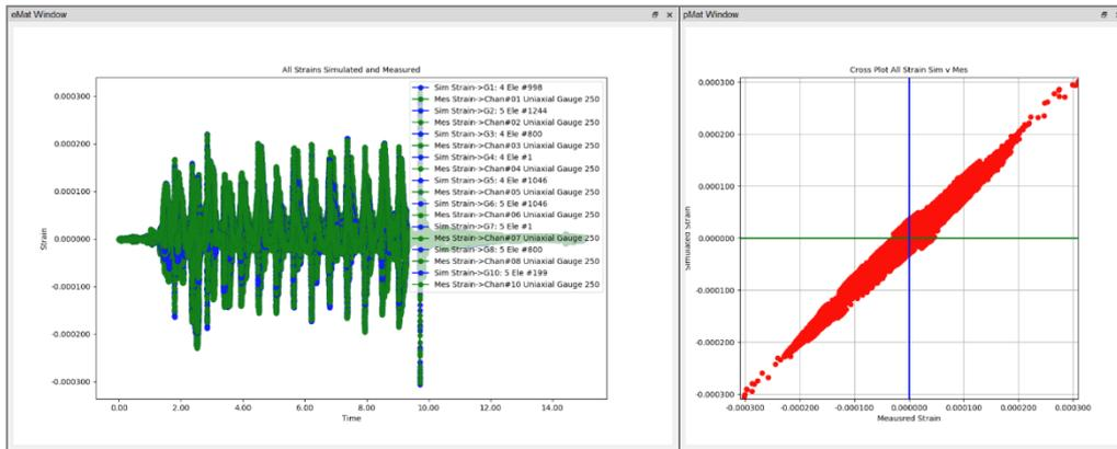
Figure 4-14 Overall Strain Correlation Plot
