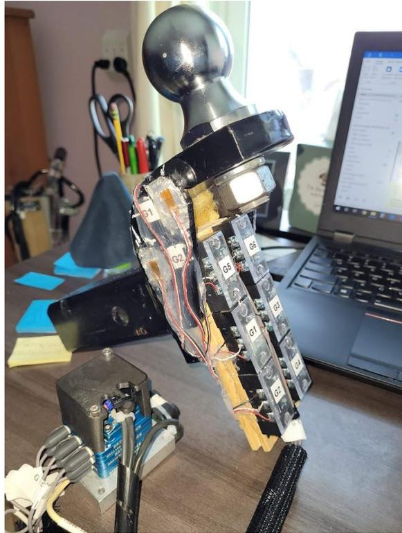
Figure 5: Strain Gauge Placement
