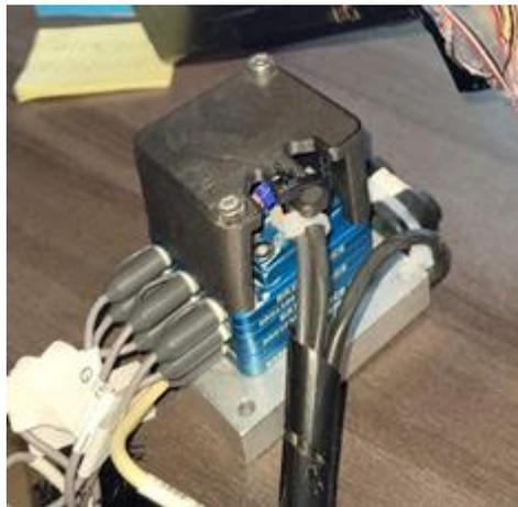
Figure 11: DAQ used for Strain Data Collection
